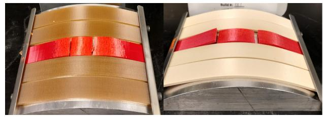
Figure 8: Non-annealed (left) and annealed (right) specimens after exposure to Ethyl Acetate (orange = ULTEM™ 9085 resin)
