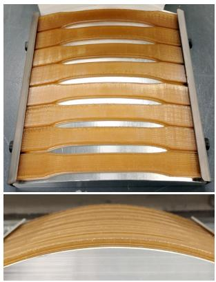
Figure 3: Non-annealed Antero 800NA ZX tensile samples in 1% strain fixture pre-exposure.
