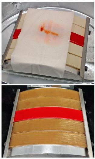
Figure 5: Visual testing Antero 800NA vs. ULTEM™ 9085 resin (orange) set-up (annealed – top, non-annealed – bottom).
