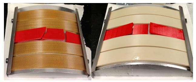
Figure 7: Non-annealed (left) and annealed (right) specimens after exposure to Skydrol (orange = ULTEM™ 9085 resin)
