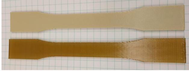
Figure 1: Annealed (top) vs. non-annealed tensile specimens.
