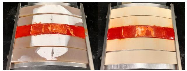
Figure 10: Non-annealed (left) and annealed (right) specimens after exposure to Dichloromethane (orange = ULTEM<sup>TM</sup> 9085 resin)
