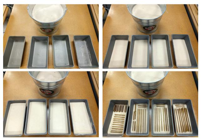
Figure 2: Samples should be placed in a sand bath to prevent deformation while being annealed.
