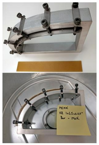
Figure 2: Variable Strain Fixture - shows the extent of deformation under various strains with chemical exposure. Some samples broke above 1% strain with certain chemicals.
