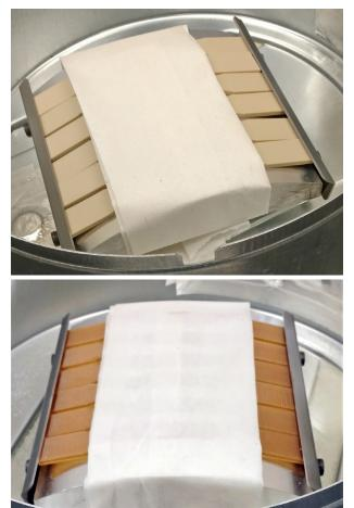
Figure 4: Tensile 1% strain test set-up - cloth in position across test area (annealed – top, non-annealed – bottom).
