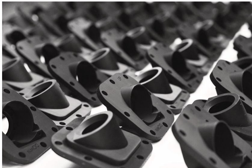
The Stratasys Origin One 3D printer is designed for mass production applications, such as these camera housings.
