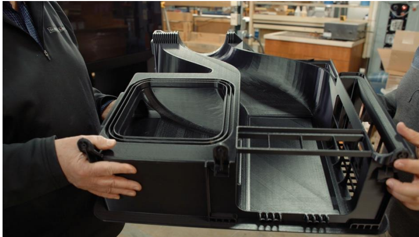
Luxury appliance manufacturer Sub-Zero Group harnesses the F770 3D printer for parts that were previously too large to produce in-house
