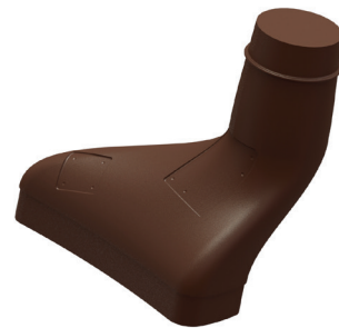
Figure 4-3: Extending open faces and adding trim lines and locating features assist in the lay-up and post-processing of the composite part.
