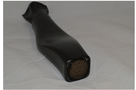
Figure 7-2: Shrink tubing is a simple consolidation method that can be used for specific geometries.
