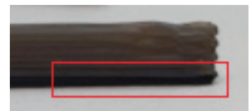
Figure 5-12: Two layers of ST-130_S support material are automatically generated underneath the stabilizer wall, ensuring that it adheres to the build sheet.
