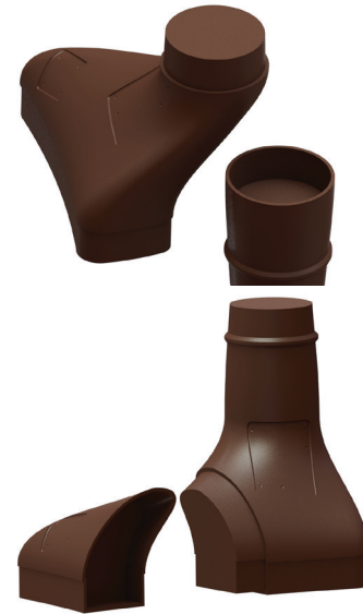
Figure 4-6: Tools that are larger than the build chamber of the machine must be sectioned in CAD.
