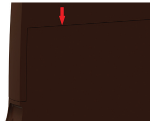
Figure 4-7: A 0.005 inch clearance between each face (a total of 0.010 inch) of components is recommended.
