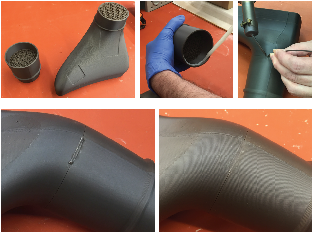
Figure 4-8: Sectioning tools in CAD and bonding them together post-build using hot-air welding and/or epoxy allows for production of tools larger than the build chamber of the FDM machine.
