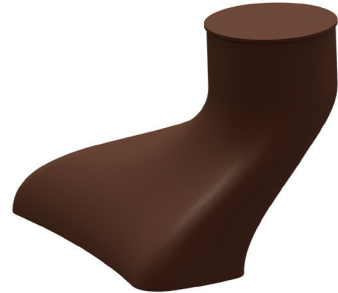
Figure 4-2: A solid body is created by extracting the interior surface of the composite part by closing open areas (top). Hiding the composite part reveals the sacrificial tool (bottom).
