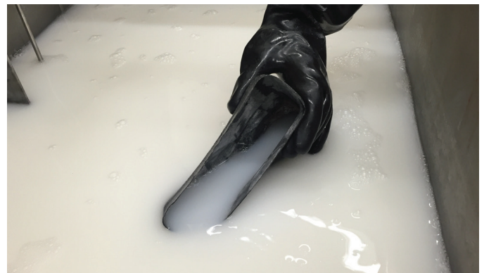
Figure 10-2: FDM sacrificial tooling easily washes out in a detergent solution.
