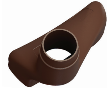
Figure 4-4: An additional shelling step creates a shell tool from a sparse tool.
