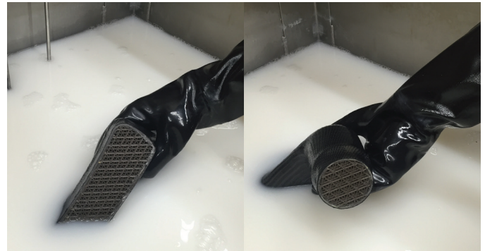
Figure 10-1: Tooling faces without composite material should be broken open or built without cap layers to promote fluid flow through the tool.
