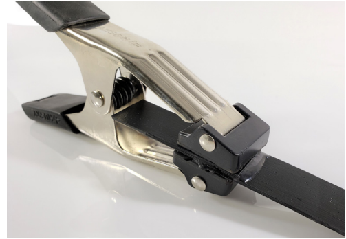
Figure 13: Clamping the pieces while the adhesive sets
