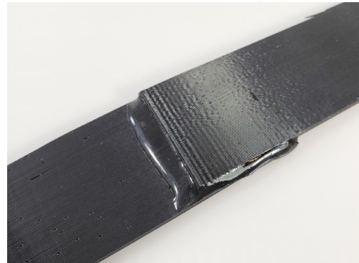
Figure 14: Bonded area after the adhesive is fully cured
