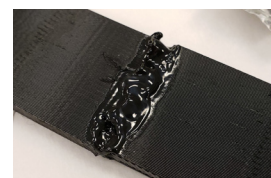
Figure 8: Welding with hot air
