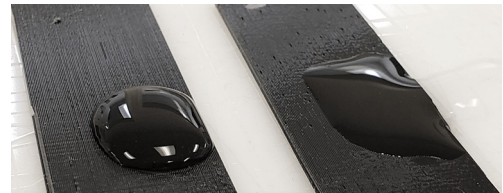
Figure 11: Surface energy before (left) and after sandblasting (right)
