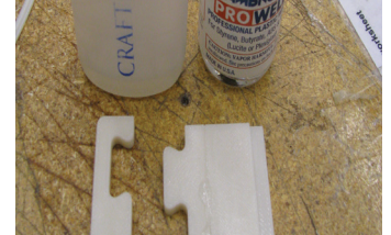
Figure 15: The low-viscosity solvent also flows well into seams and cracks.
