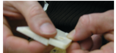
Figure 16: Align and hold the mating piece until the bond has set.
