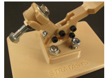
Clamping device with a variety of mechanical fasteners.
