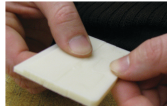
Figure 8: Hysol E-20HP epoxy has good bond strength and chemical resistance.
