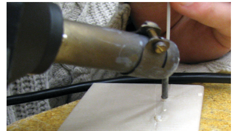
Figure 17: Hot air plastic welding is similar, in concept, to oxy-acetylene welding.
