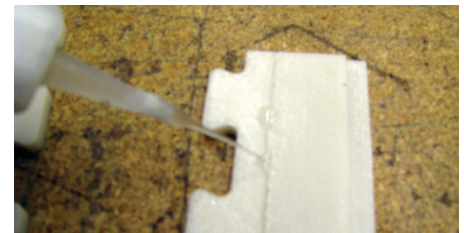
Figure 4: Apply cyanoacrylate to mating surfaces.
