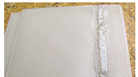
Figure 19: Bonded pieces before sanding the weld bead flush to the surrounding surfaces.
