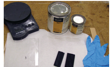
Figure 9: Supplies for application of Hysol EA 9394 epoxy.
