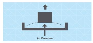
Origin's pneumatic separation mechanism applies much less separation force: the membrane gradually peels off each cured layer as the build platform goes up.
