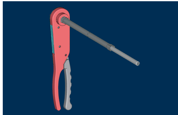
ProEngineer was used to design the surgical ratchet.
