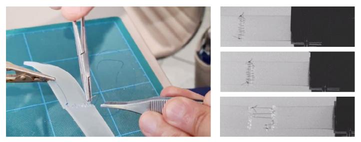
Figure 2: Uniaxial tensile test performed on a 3D printed sample sutured by an expert surgeon in order to mimic the surgical suture on a medium caliper arterial vessel
