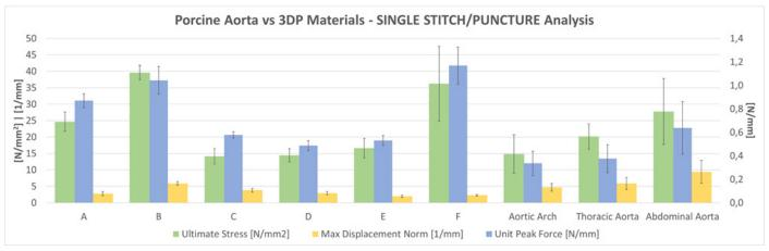
Figure 3: Overall results of puncture and single stich tests on the pool of 6 selected materials compared with porcine aorta tracts (namely aortic arch, thoracic aorta and abdominal aorta).
