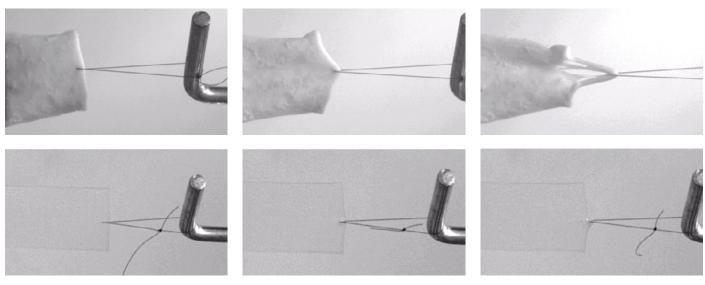
Figure 1: Comparison between single stitch mechanical tests performed on porcine aorta (up) and on a 3DP material (down).
