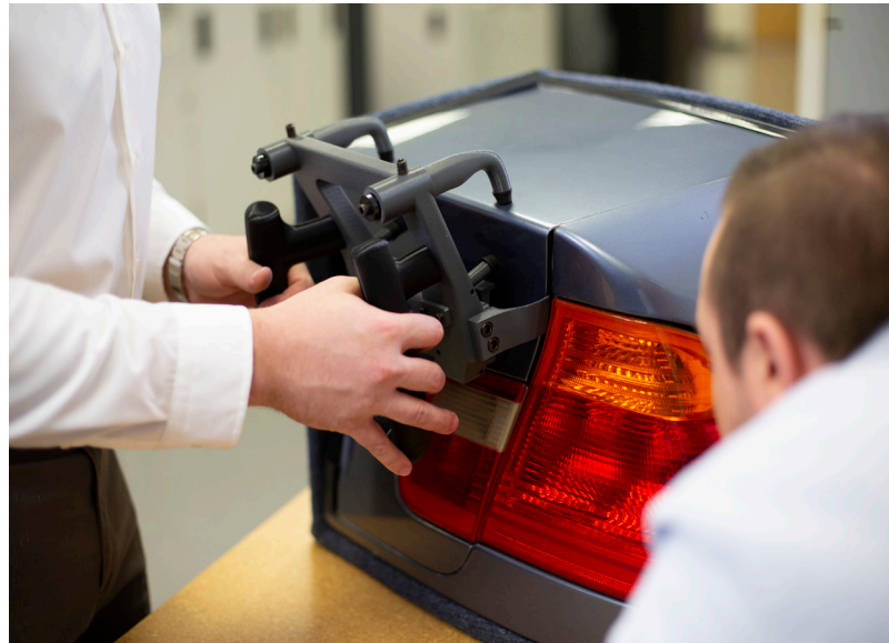
Figure 3 – 3D Printed Jig being used for an automotive part.
