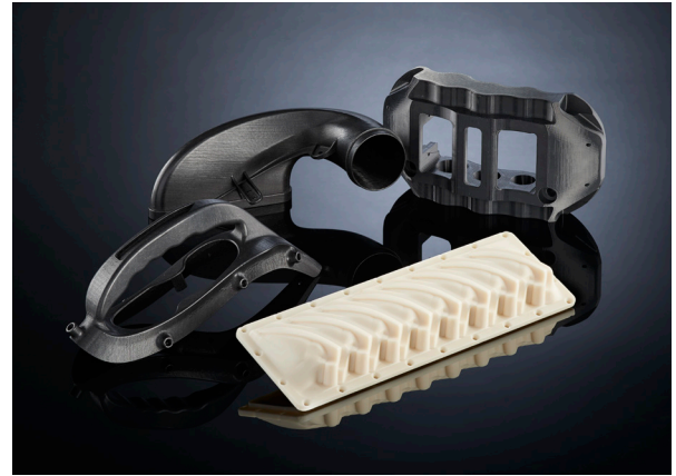
Figure 1: Production grade FDM parts printed using the Stratasys Fortus380mc
